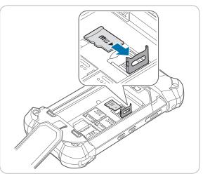
3 Lift down the fasteners and slide it to left for locking the slot.
