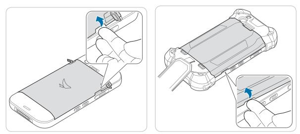
When removing the battery cover, be careful not to damage your fingernail.
