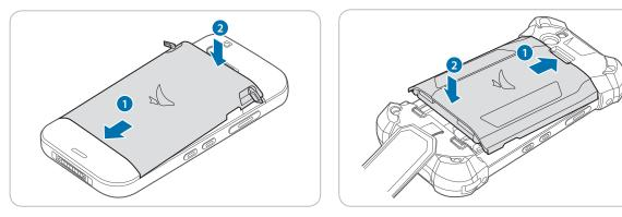
5 For the EF500 device, close the battery locks to lock the battery cover. For the EF500R device, slide up the battery locks to lock the battery cover.
