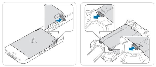
2 Use the notch and lift the battery cover. Remove the cover completely.
